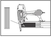
Figure 2. Loading the nailer.
